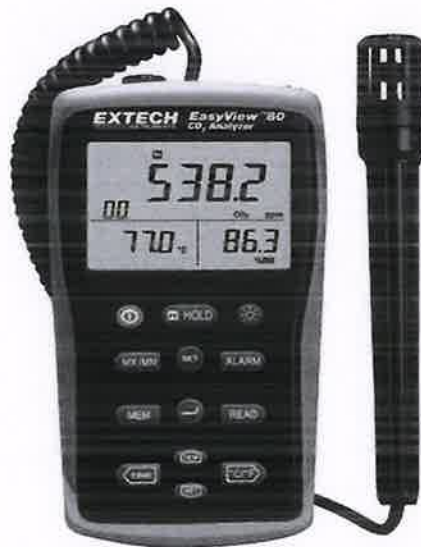
Figure 6. Indoor air quality meter
